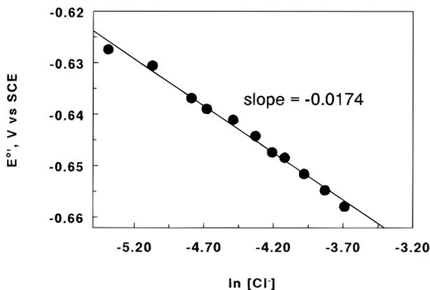
**Figure 2.** Influence of chloride ion concentration on the formal potential of PLL- $\text{B}_{12}(\text{COOH})_6$  film in an aqueous 5 mM TRIS buffer, pH 7.1.
