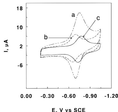
**Figure 1.** Cyclic voltammograms of PLL-B<sub>12</sub>(COOH)<sub>6</sub> film at 50 mV s<sup>-1</sup> in (a) pH 7.10 TRIS buffer in water, (b) SDS/pentanol/dodecane/water microemulsion **3**, and (c) CTAB/hexadecane/pentanol/water microemulsion **9**.
