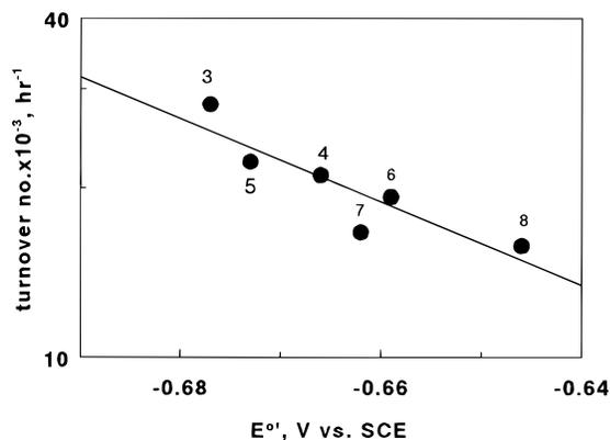
**Figure 8.** Influence of the formal potential of PLL-B<sub>12</sub>(COOH)<sub>6</sub> films on the logarithm of turnover number from catalytic electrolyses of DBCH in bicontinuous SDS microemulsions. (The numbers near points identify microemulsions in Table 1.)
