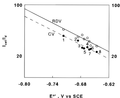
**Figure 6.** Influence of the formal potential of PLL-B<sub>12</sub>(COOH)<sub>6</sub> films in SDS microemulsions on the voltammetric catalytic efficiency  $I_{\text{cat}}/I_a$  from CV and RDV at 50 mV s<sup>-1</sup>. (The numbers near points identify microemulsions in Table 1.)
