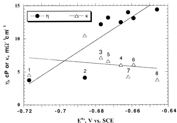
**Figure 7.** Correlation plots of viscosity and conductivity of microemulsions against  $E^{\circ'}$  of PLL-B<sub>12</sub>(COOH)<sub>6</sub> films. (The numbers near points identify microemulsions in Table 1.)
