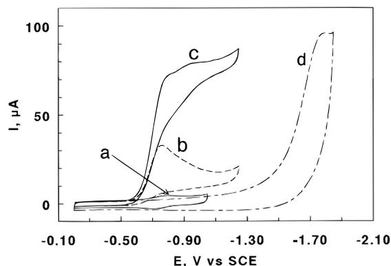
**Figure 5.** Representative voltammograms of PLL-B<sub>12</sub>(COOH)<sub>6</sub> film at 50 mV s<sup>-1</sup> in microemulsion 1: (a) CV with no DBCH; (b) CV with 7 mM DBCH present (second scan); (c) RDV with 7 mM DBCH present; and (d) direct CV reduction of 7 mM DBCH on the PG/PLL electrode.
